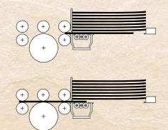
All other feeders stop feeding here, causing excessive feed roll grip (crush) in order to remove the sheet from the stack.
